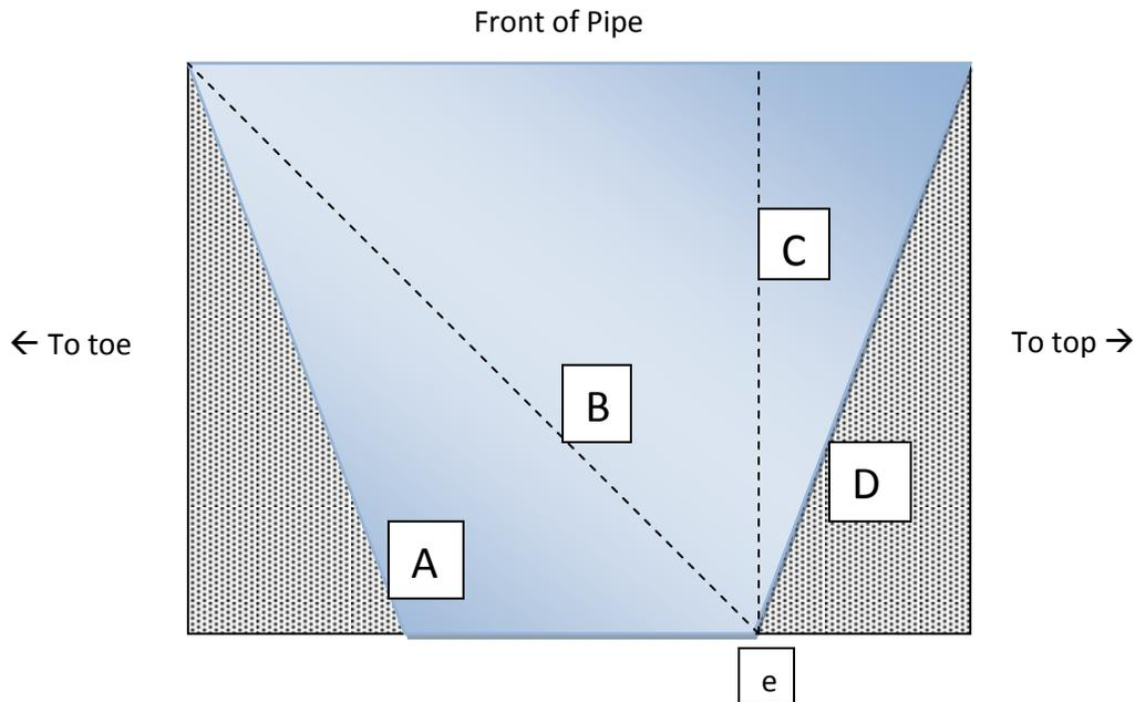
The blue shaded area is the wedge, which is a trapezoid (specifically, it is an Isosceles trapezoid, which means it is symmetrical—the side legs are both the same length). The gray shaded areas are there just to aid understanding.
