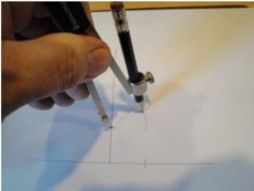
Figure 10 - Draw an arc from the mark to the inside of the angle
