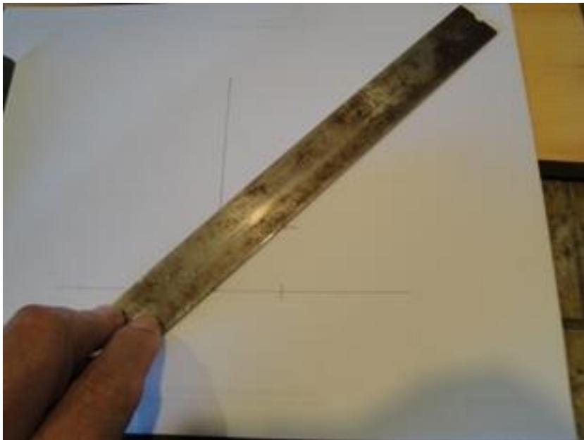
Figure 12 - Draw a line from the origin through the intersection of the two arcs
