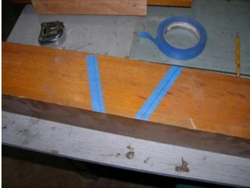
Figure 2 - Both cut lines are marked and ready to saw
