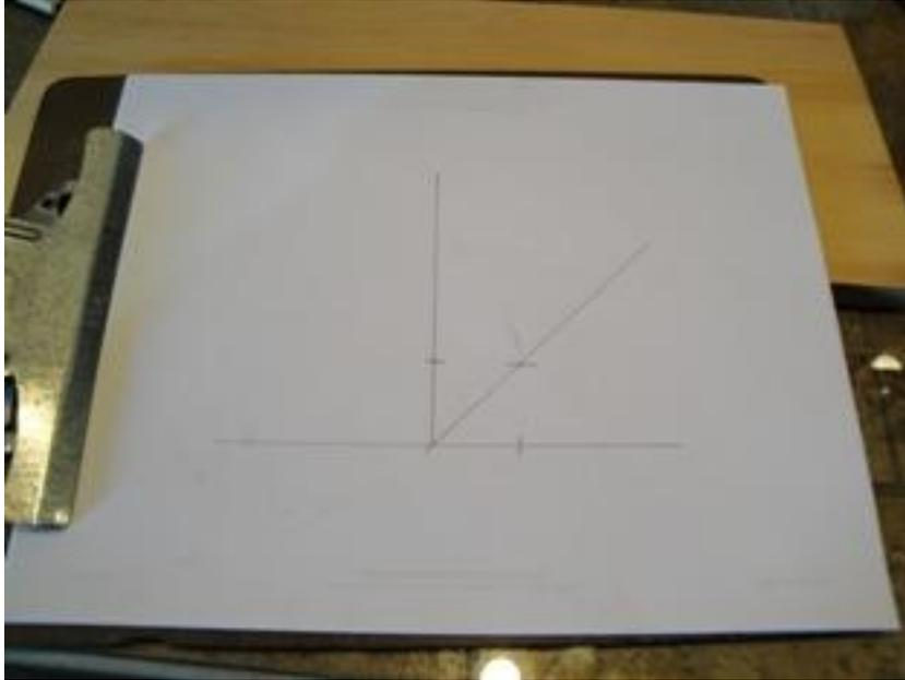
Figure 13 - You now have a  $45^\circ$  angle. Follow the same steps again, using the  $45^\circ$  ray, and you can create a  $22\frac{1}{2}^\circ$  angle
