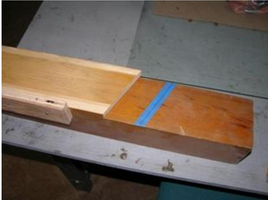
Figure 8 - A simple template for laying out  $22\frac{1}{2}^\circ$  lines
