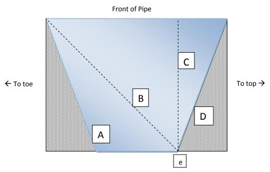
The blue shaded area is the wedge, which is a trapezoid (specifically, it is an Isosceles trapezoid, which means it is symmetrical—the side legs are both the same length). The gray shaded areas are there just to aid understanding.
