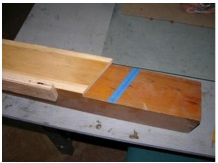
Figure 8 - A simple template for laying out 22½° lines
