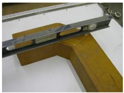
Figure 1 - The bottom of the mitered section aligns with the top of the cut at the back of the pipe. That's why the dimensions of the wedge are important. If the wedge was either larger or smaller, the alignment (and visual effect) would be off.
